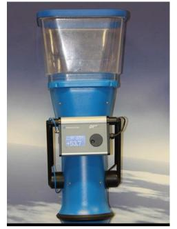
As soon as the zero-pressure state is achieved, which is normally between 4 and 20 seconds, the instrument displays the air volume flow rate. Some instruments may also display the air temperature.
