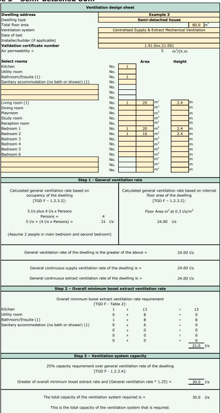
The total supply airflow rate of 24 l/s must be delivered to the habitable rooms in proportion to their volume. In this example the general ventilation rate > Overall minimum boost extract ventilation rate.
