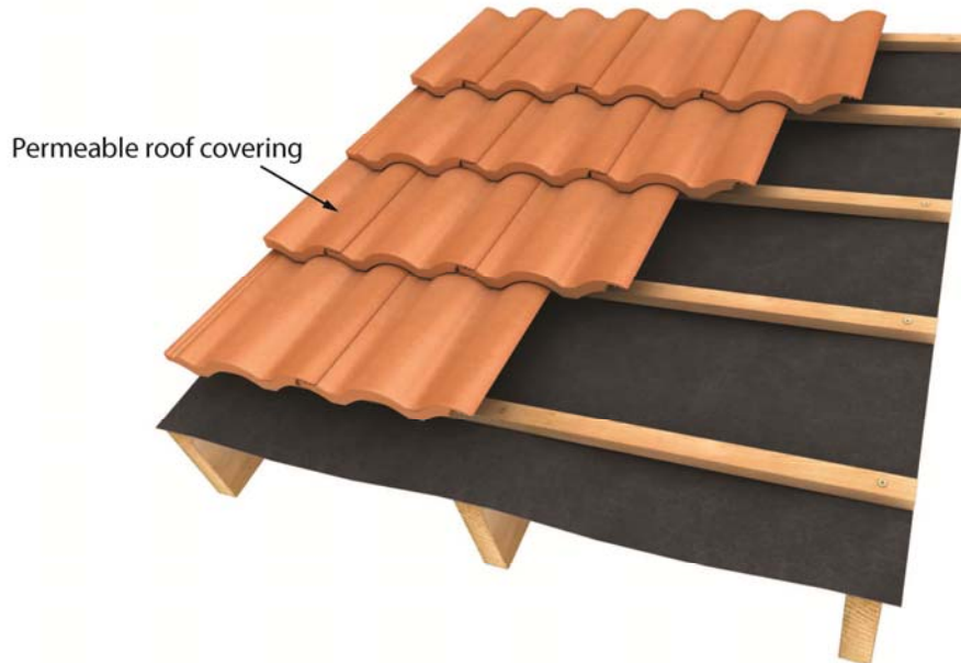
Figure 1: Cold Roof detail with permeable roof covering
