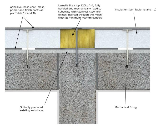
Figure 4: Fire Break Detail
