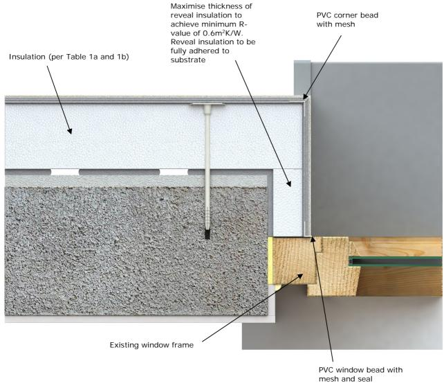
Figure 3: Window Reveal Detail
