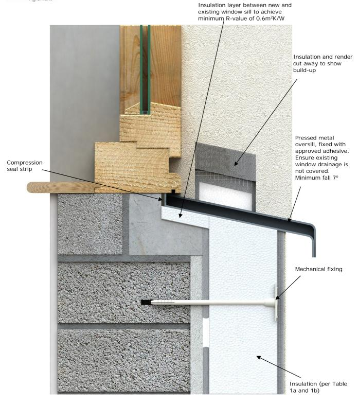
Figure 2: Window Sill Detail
