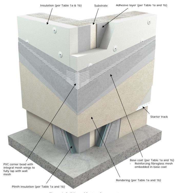
Figure 1: Build-up of System Components
