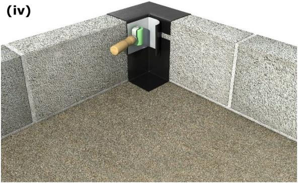
Cut another section of Monarseal MRX tape to join the L-cap to the internal section (Ensure a lap of 50mm to each piece). Use a hand-roller to complete seal.
