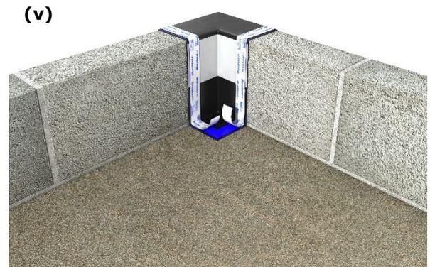
Apply a strip of Monobond RT double-sided tape to each edge of the corner assembly.
