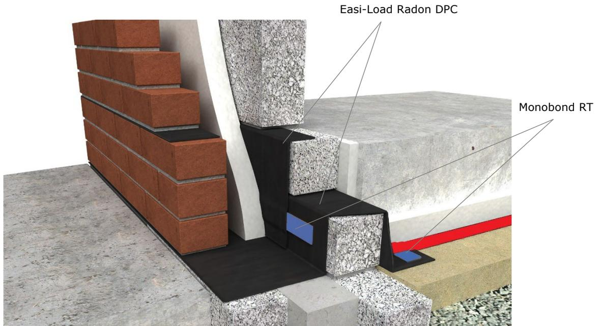
**Figure 8: Detail showing Monarflex® radon membrane and Easi-Load under floating slab**
