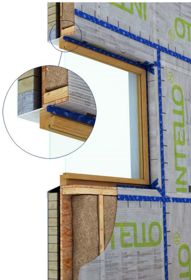
Figure 2: Window Detail sealed with TESCON PROFIL
