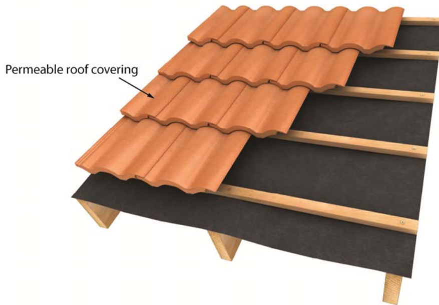
Figure 1: Cold Roof detail with permeable roof covering
