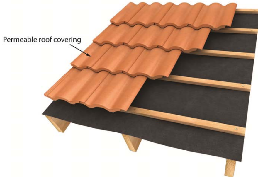
Figure 1: Cold Roof detail with permeable roof covering
