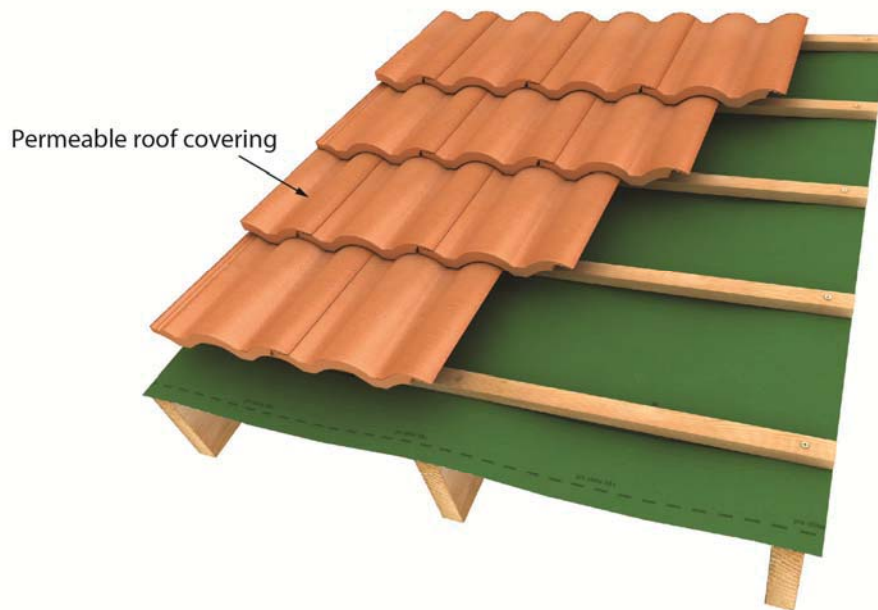
Figure 1: Cold Roof detail with permeable roof covering
