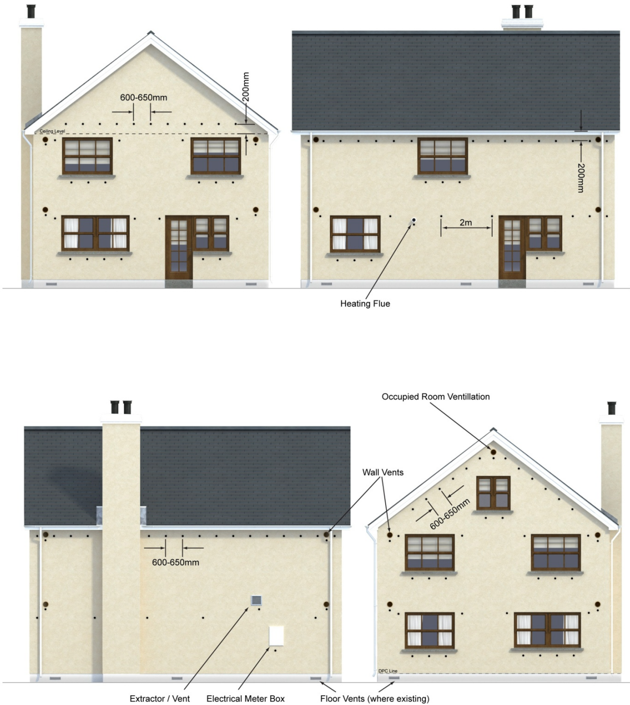
Figure 1: Typical Energystore Hole Drilling Pattern in a Detached Dwelling New and existing buildings without existing partial fill insulation in cavity.
