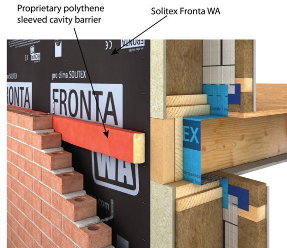
Figure 4: At Cavity Barriers
