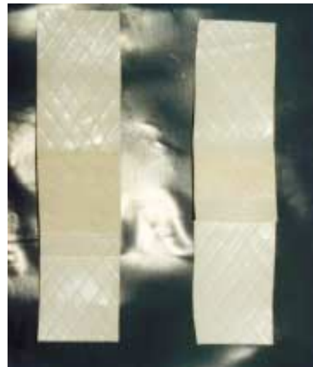
Fig1B: Close up view of factory sealed fusion joint
