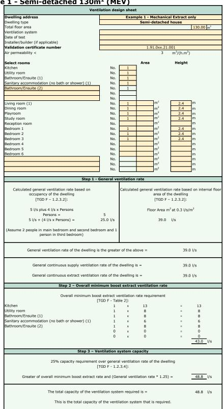
Extract should be from each wet room and sanitary accommodation. The continuous extract ventilation rate at each extract point is adjusted proportionally.
