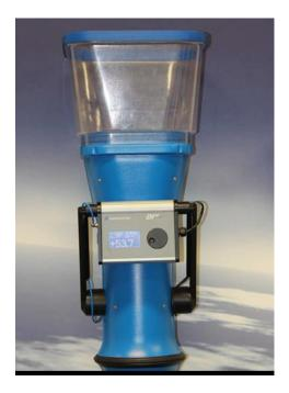
As soon as the zero-pressure state is achieved, which is normally between 4 and 20 seconds, the instrument displays the air volume flow rate. Some instruments may also display the air temperature.
