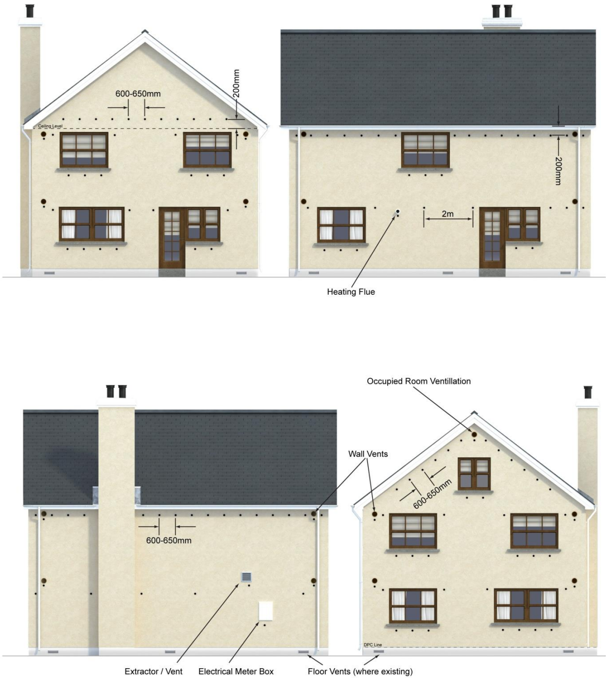
Figure 1: Typical Thermobead Plus Hole Drilling Pattern in a Detached Dwelling. New and existing buildings without existing partial fill insulation in cavity.
