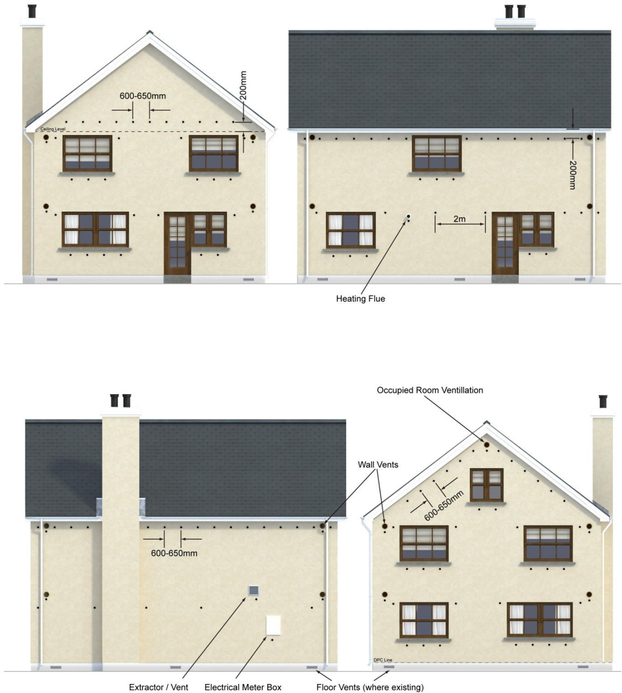
Figure 1: Typical Envirobead Hole Drilling Pattern in a Detached Dwelling. New and existing buildings without existing partial fill insulation in cavity.
