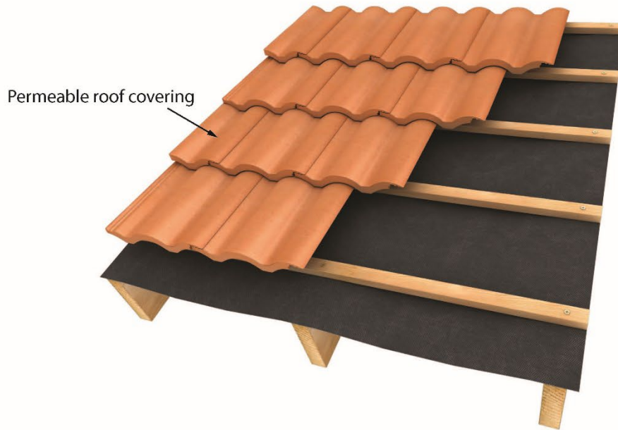
Figure 1: Cold Roof detail with permeable roof covering
