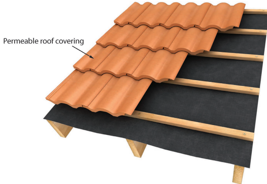
Figure 1: Cold Roof detail with permeable roof covering
