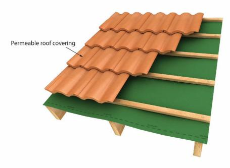
Figure 1: Cold Roof detail with permeable roof covering
