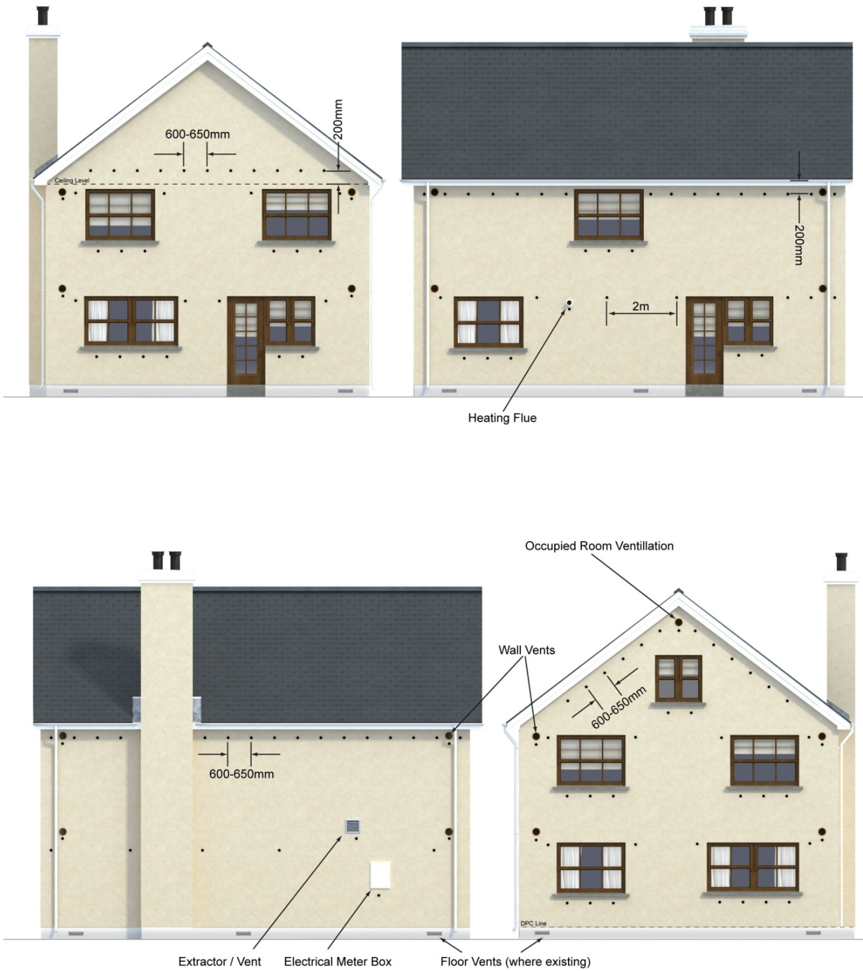
Figure 1: Typical Kingspan EcoBead Hole Drilling Pattern in a Detached Dwelling New and existing buildings without existing partial fill insulation in cavity.
